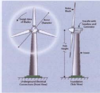
Drawing of the rotor and blades of a wind turbine, courtesy of ESH
